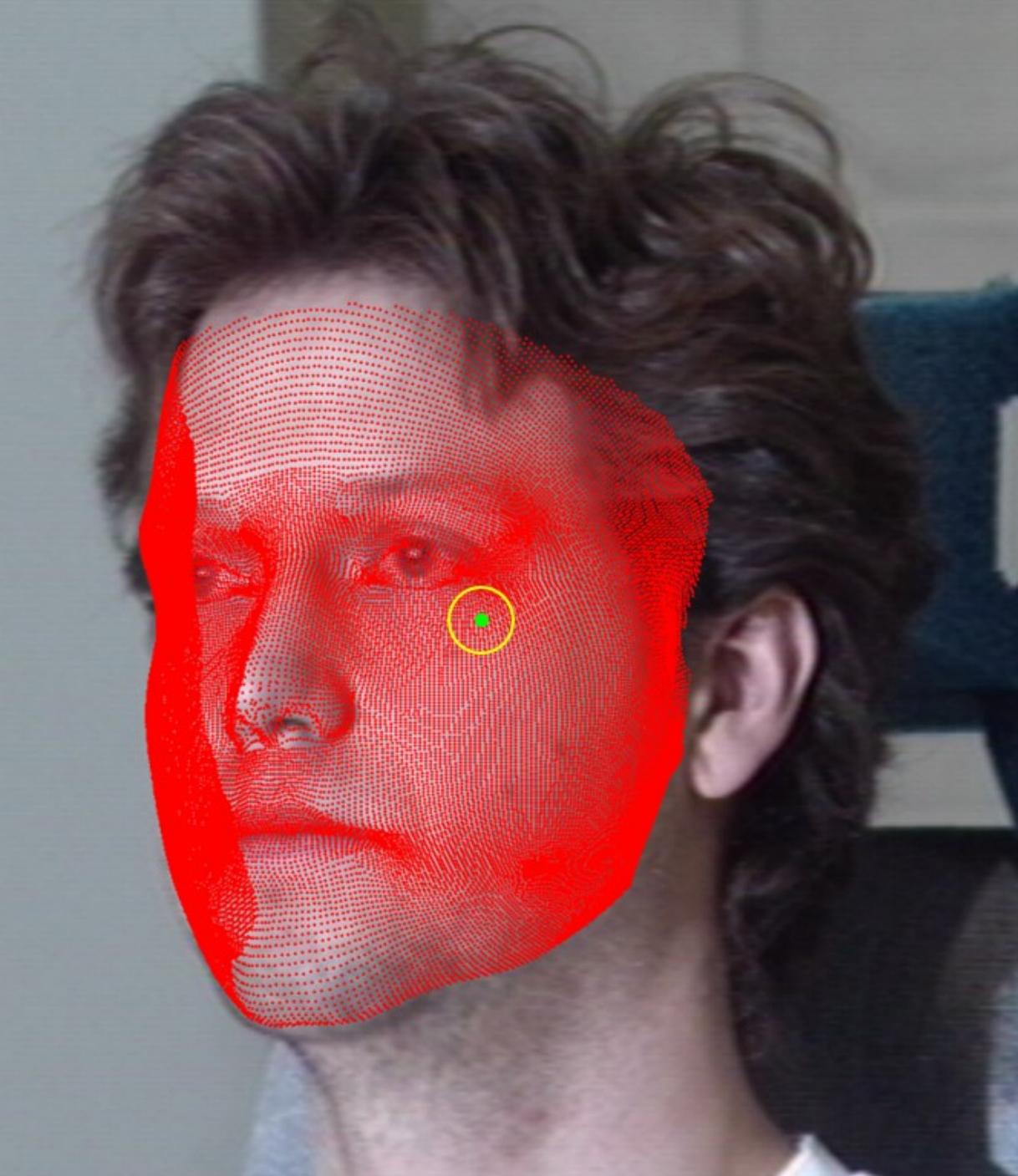
**Figure A.6:** A single vertex projected onto the image plane is shown in green. To determine if this vertex is occluded by other parts of the 3D model, we only need to check for intersections with the triangles made up of vertexes in the yellow circle. Anything outside this would be too far away to occlude the point given the density of the model.
